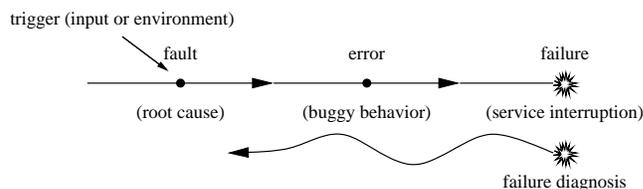
Figure 1: Failure diagnosis is driven by occurring failures and tries to understand the whole fault chain
