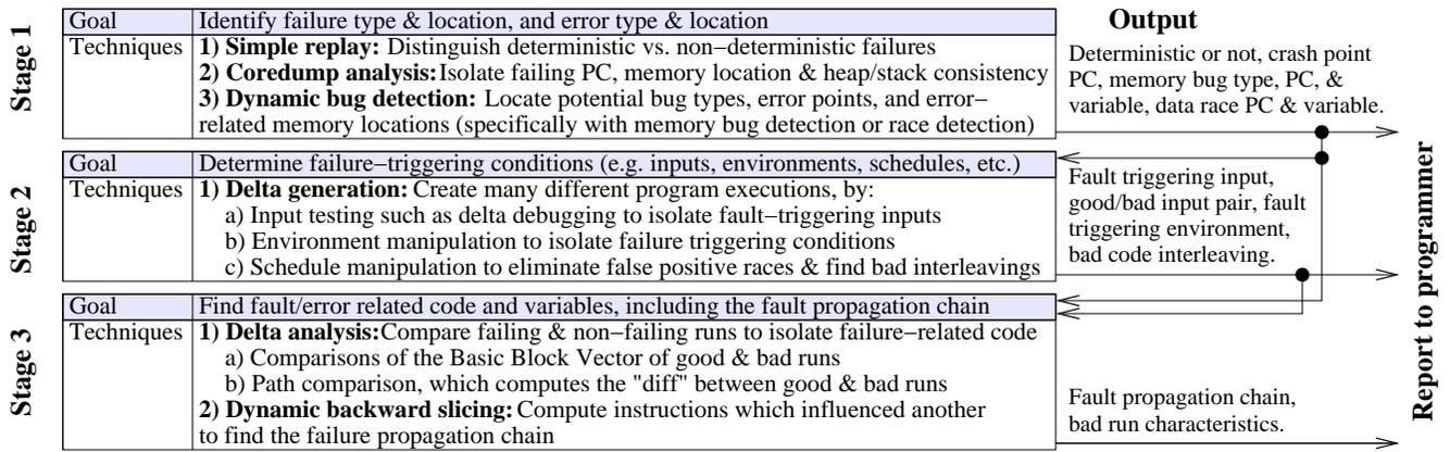
**Figure 3: Diagnosis protocol (TDP) diagram** (This figure illustrates the Triage diagnosis protocol, including the failure diagnosis components we have implemented. These separate analysis components are run in one or more iterations of reexecution, during which all side-effects are sandboxed. Later stages are fed results from earlier stages as necessary.)
